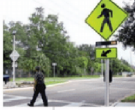
Rapid Flashing Beacon
